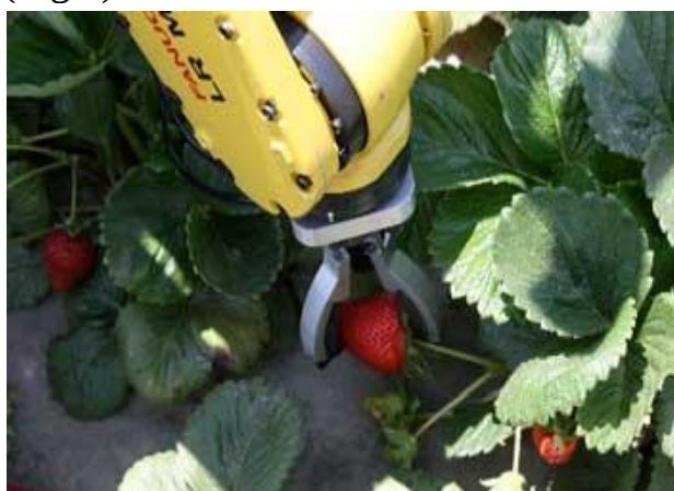
Fig.2 – Capture robotics hand with berries
