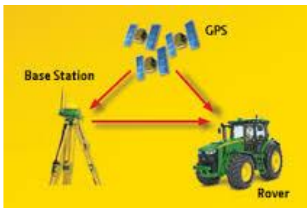
Fig.3 – Schematic diagram of the automatic driving of the tractor
