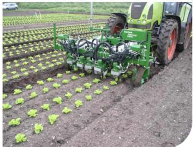
Figure: 5 Robocrop InRow Weeder
