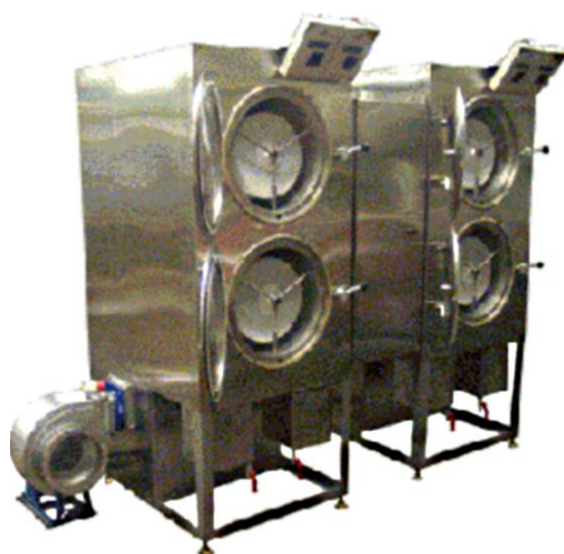
Figure 2.8 - Microwave vacuum unit "Musson" [40]
